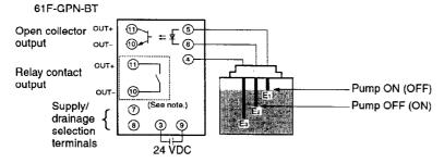
Note: The part within the dotted-line box is for the 61F-GPN-BC (relay-output type) only.
